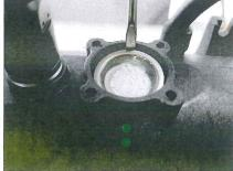
12. Check under where the cup sits for debris and any damage to the tube.
