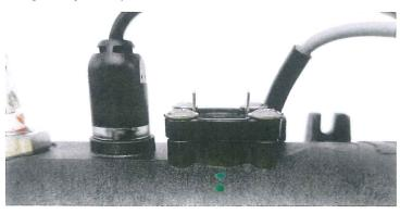
21. Remove the earth screw and place the earth wire onto the element and screw it down tight.
