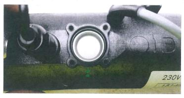
17. Place O-ring 1 onto the retaining plate. Make sure that it is not twisted and is sitting flat. Fit the thermal overload into the retaining plate. As the plate is moulded to the thermal overload shape the thermal overload only goes in one way.
