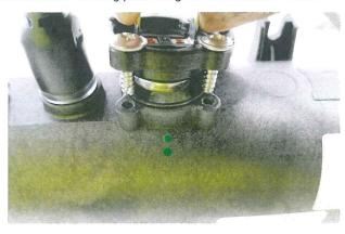
11. Now the thermal overload cup can be seen. Remove the O-ring that sits between the retaining plate and this cup. Gently lift the cup using the Small Flat Blade Terminal Screw Driver and remove.
