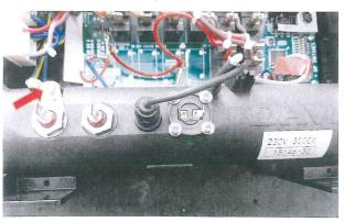
22.Lift the tube up and place it on an angle so that you can slide the tube retaining tab under the upper screw.
